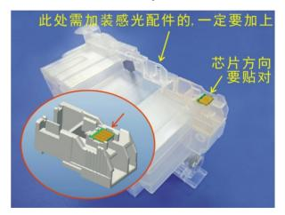
5. stick the double-sided adhesive 6. stick the chip on the position as on the chip show
