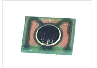
3-4. you can see it have some residue on the chip when you teardown so must be make it clear, but don't broken the chip.
